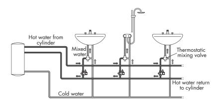
Before fitting the thermostatic balancing valve, the pipes must be thoroughly flushed to remove any debris or particles which will reduce it's performance.
